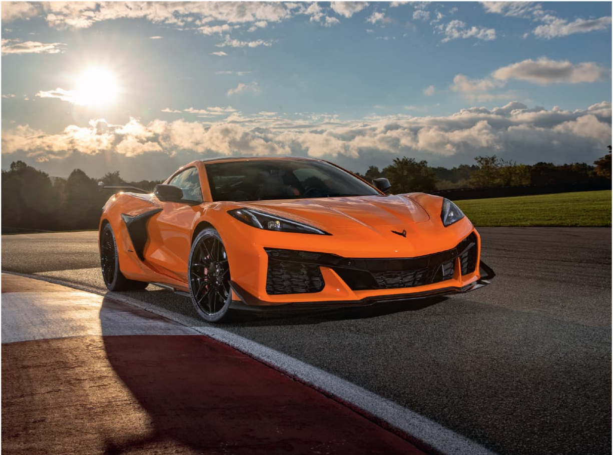
The Z06 body measures 3.6 inches (9 centimeters) wider than a Stingray. The added width accommodates wider tires, improves aerodynamic performance, and delivers a far more aggressive stance
