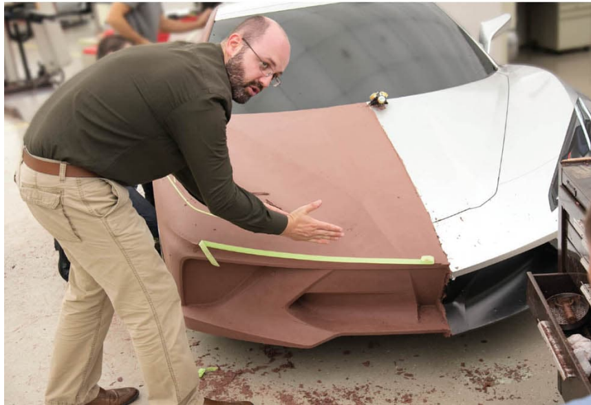
Exterior designer Hwasup Lee (previous photo) and Vlad Kapitonov (above) examine the shapes that came out of the new architecture—which not only act as guides for airflow, they also echo key design cues long associated with Corvette.
