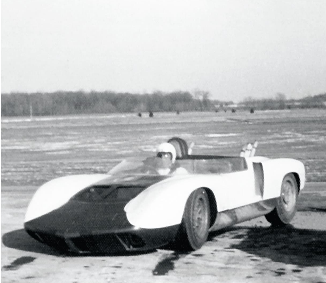
The CERV II race car had two transmissions—one for the front wheels and one for the rears. The GS IIb was Chevrolet R&D boss Frank Winchell's idea.
