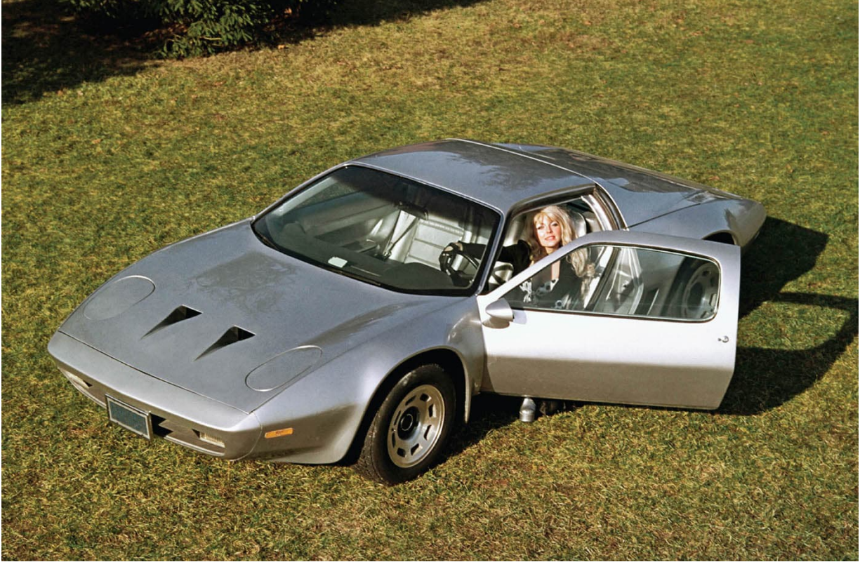
XP-895, also known as the Reynolds Aluminum Corvette. The concept car's body broke with the tradition of Corvettes having fiberglass bodies, which they had since Day One.
