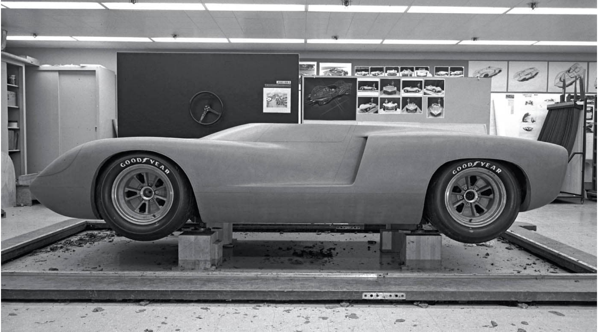
The CERV II concept begins to take shape as this clay model in Chevrolet's Advanced No. 3 Studio.
