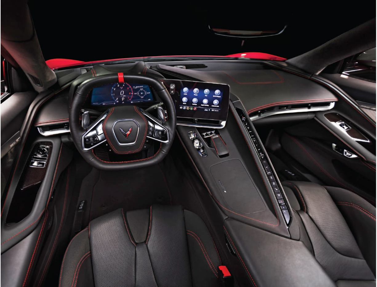
The passenger compartment moves forward a whopping 16.5 inches. Forward visibility is much better, thanks to a much lower cowl and instrument panel.
